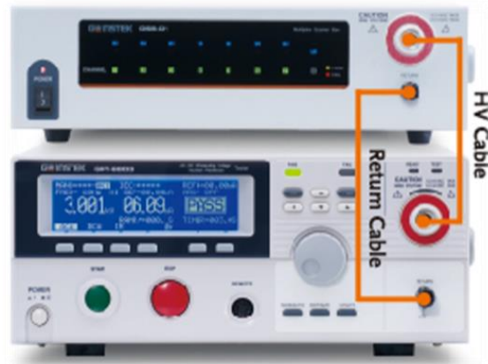
(b) External multiplex scanner box: GPT-9000 series
