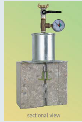
Figure 2: Set-up with terminal for the pressure-water test
