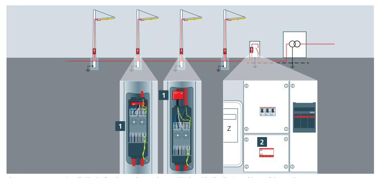
The surge arresters are installed in the fuse box at the mast base and in the cable distribution cabinets of the supply system.
