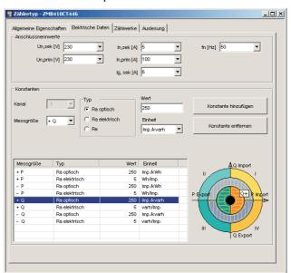
The basic version supports the communication protocol in accordance with that described in the IEC 62056-21 Mode C standard. As an additional option the communication protocol is prepared according to dlms / COSEM.
