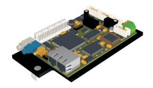
**SMM 400 Bus-Master** provides the interface between personal computer (via ETHERNET) and the system modules over RS 485-Ringbus.
