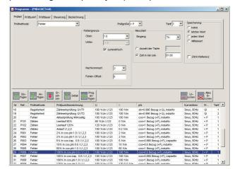
In addition to the respective test method (e.g. error measurement, register tests, ...) each checkpoint can be linked with control commands. Control commands display for instance instructions to the operator, switching of tariff relays or dispatching of commands e.g. to adjust time, ...
