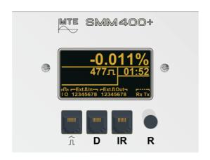
**SMM 400+** Meter Evaluation Module with full graphic OLED display, reset-button and 2 scanning head pulse inputs is the perfect solution to test modern meters.
