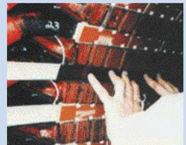
*Iris Power Stator Slot Coupler Installation in a stator slot.*
