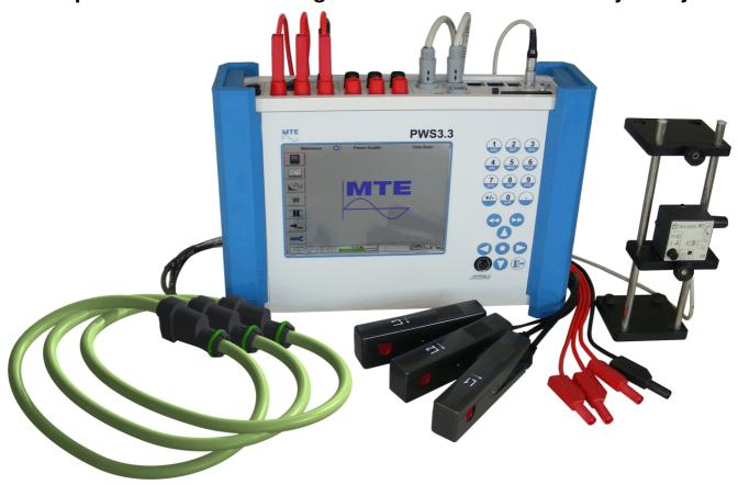
The PWS 3.3 is a combination of a three-phase Portable Working Standard of class 0.05% or 0.1% and an IEC 61000-4-30 Class A compatible Power Quality Analyzer with 3 voltage and 4 current channels.
