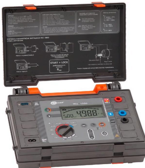
MIC-5000 tester is designed to measure insulation resistance of power cables, transformers, motors and other electrically powered devices. Additionally the device allows for measurement of AC and DC voltages. Input circuits of the measuring devices are electronically protected from overloading, e.g. due to incorrect connection to the circuit being tested or incorrect use of input terminals.
