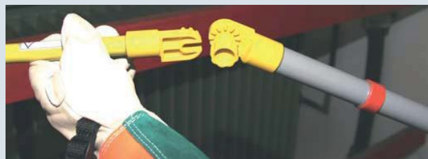
The universal gear coupling permits fast replacement of operating heads and extensions
