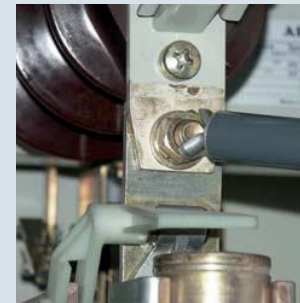
Testing with screwed-on V-shaped electrode
