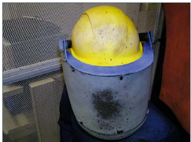
Safety helmet for electricians with face shield protects the face and head region from injuries and burns.
