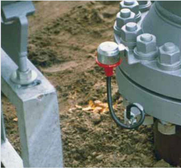
ATEX and IECEx-certified isolating spark gap for lightning equipotential bonding according to IEC 62305 with flexible conductor connection
