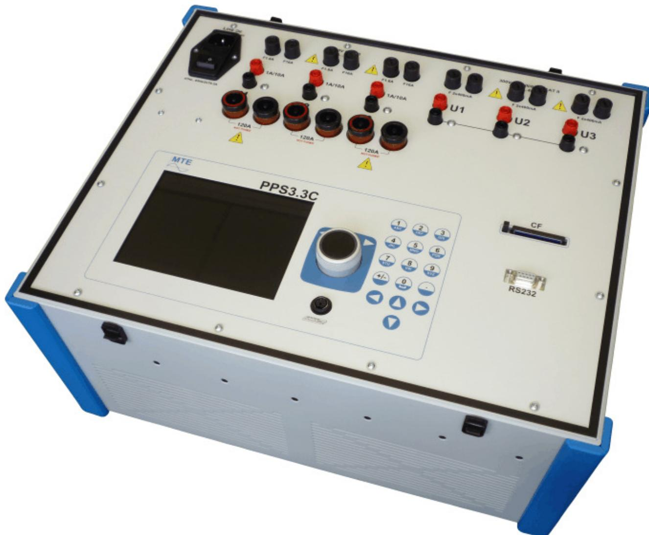
The PPS 3.3 C is a powerful and portable three-phase current and voltage source. All test values are generated absolutely synthetically with a high degree of accuracy and stability.
