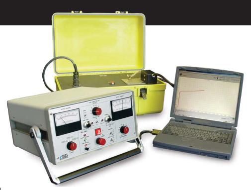
The Iris Power DCR 50™ is a simple off-line DC tester to identify problems in the stator groundwall insulation system of large AC electric machines before an unexpected in-service failure occurs. Unlike the pass or fail of a DC or AC hi-pot test, the DC ramp test gives diagnostic information and often can be stopped before a failure occurs.
