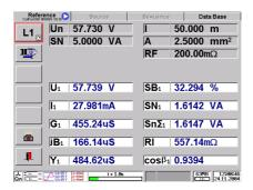
Burden measurements are carried out on the secondary side of the current and voltage transformers.
