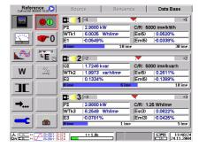
CALPORT 300 makes it possible to simultaneously test up to three electricity meters with varying constants (e.g. master and check meter of a 0.2S metering installation). Another option is a parallel test using the scanning head and the emitting contact output.
