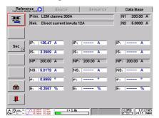
CALPORT 300 carries out these examinations by simultaneously conducting primary and secondary current measurements. Primary testing is carried out with error compensated clip-on CTs for current up to 100 A, 1000 A or flexible CTs type FLEX 3000 (for currents up to 30 A, 300 A and 3000 A). Secondary testing can be conducted directly or by using clip-on CTs.
