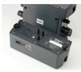
The DLRO10 and DLRO10X may also be powered from an optional mains / line power supply unit the DLRO10LPU. This unit is simply fitted to the instrument in place of the standard battery pack.
